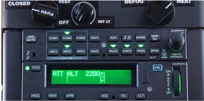
Garmin GFC 600H helicopter flight control system (HFCS)
